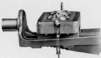
Hook Bolts Hold Mounts Securely Upon Cradle.
