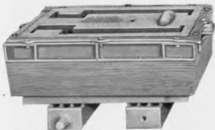
Finished cope after pattern is drawn.
